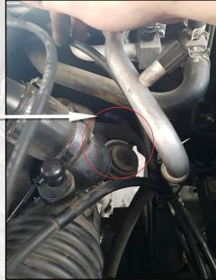
Join the two hoses removed in steps 2& 3.
